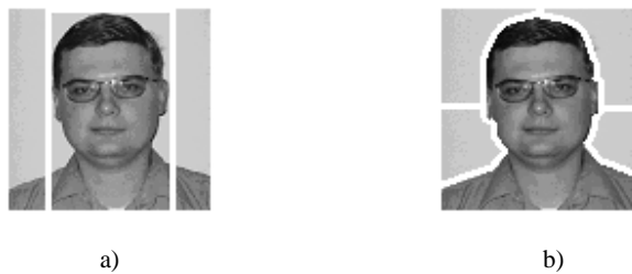
Figure 11. Test image “Slava”: (a) region of interest and (b) background four quadrant splitting.
