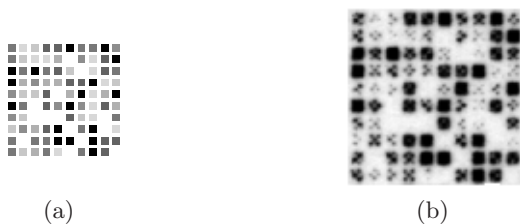
Figure 7. Eight-level 2D bar code. (a) Original digital image: 2 \times 2 pixel symbols, 1 pixel of inter-symbol space, r_i = 200 ppi. (b) Printed-and-scanned digital image: r_p = 600 dpi, r_s = 3 \cdot r_i = 600 ppi, 6 \times 6 pixel noisy symbols.
